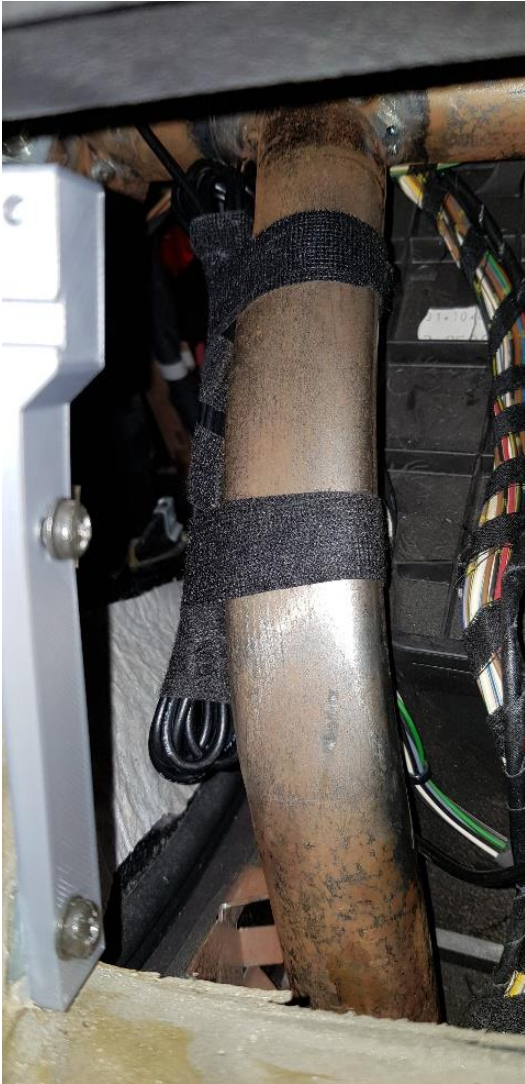
GPS receiver cable folded up and taped to steel frame
