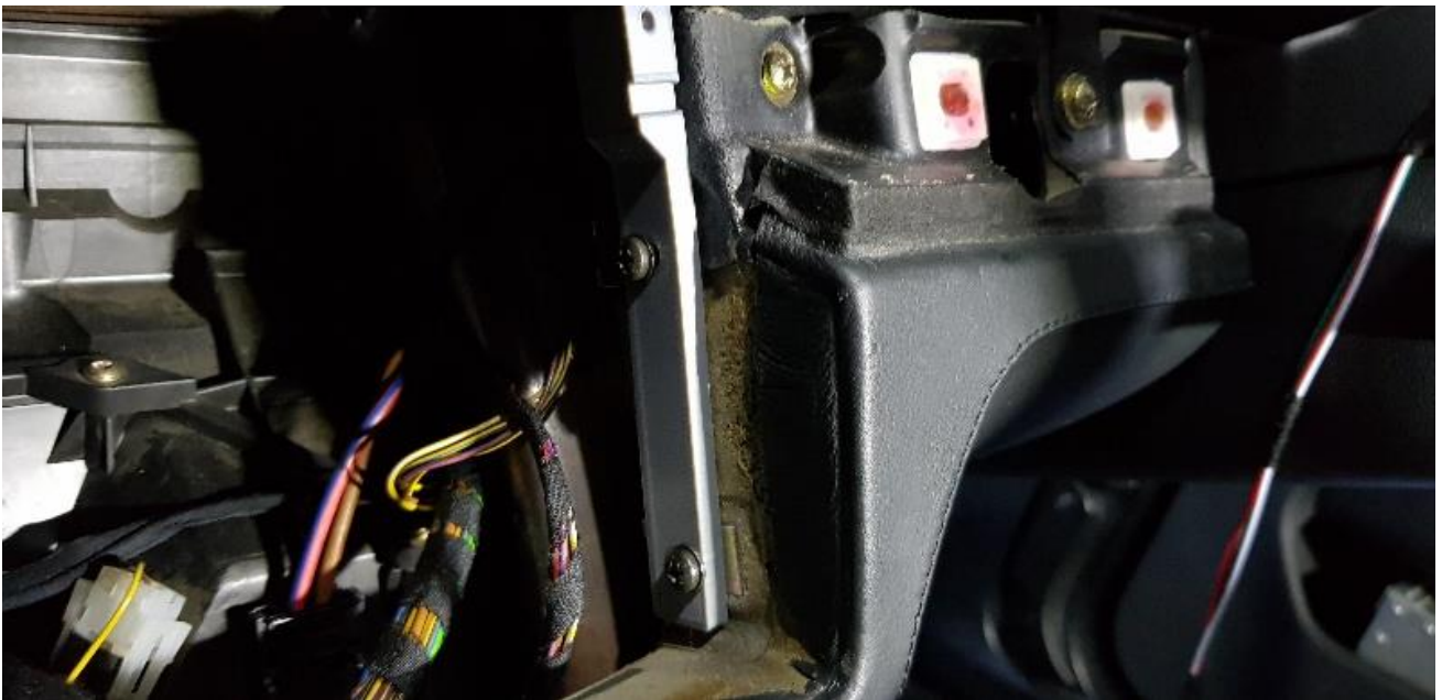
Right hand 3D printed bracket
