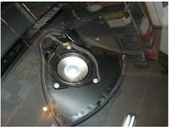
2) Using torx bit, remove 3 speaker screws.
