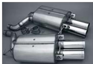
Increases power output without the excessive noise and "boominess" associated with typical aftermarket exhausts. Manufactured from 20 gauge-304 stainless steel, featuring Dinan's Tuned Resonance Chamber Technology for the optimum balance between maximum power gains and a sporty exhaust note. At just 37.6 lbs., weight is reduced by nearly 29 lbs. Dual 3" diameter polished stainless tips give the cars a tasteful performance look as well.
