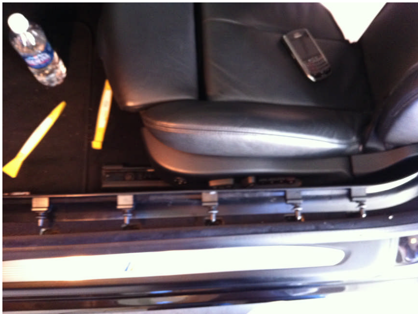
Once the trim is set aside you can spread the carpeting on the split in order to access the electrical connector
