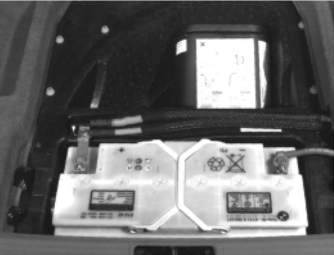
The battery is mounted, in the trunk, close to the rear bumper for weight distribution.
