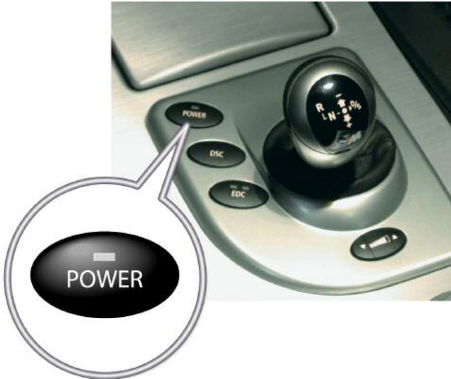
The DME receives the ground input from the switch. The SZM is responsible for the illumination of the "On" LED. Switch illumination is provided by the KL58g circuit.
