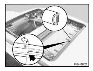
Pull off seal of sunroof cut-out at contact edge starting from body. (Peel off)
